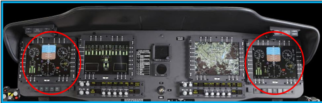
PMD - UH-60M instrument panel emulation
